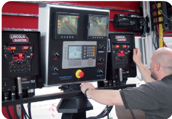
Sample view of CB operating panel and integrated SAW ACDC welding equipment from (Lincoln Electric and ESAB)
