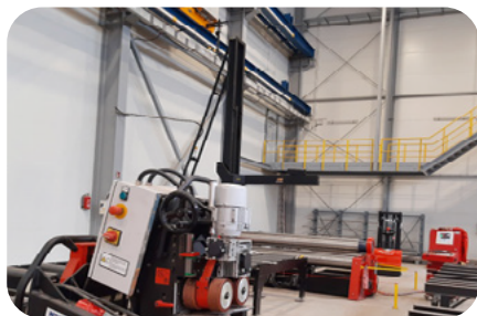
ABM-50 for high-quality single and double-sided bevels
