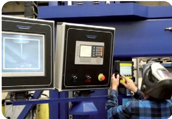
Sample view of CB operating panel and integrated MIG-MAG welding equipment from (ESAB and LORCH)
