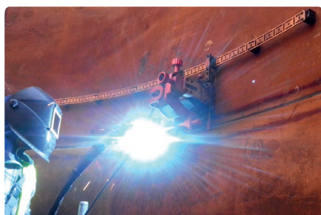
36 mm-wide flexible track, supplied in a 1.85 m (6 ft) length. Suitable for curved surfaces with a minimum radius of 1 m (3.3 ft). PRW-0466-50-01-01-0
