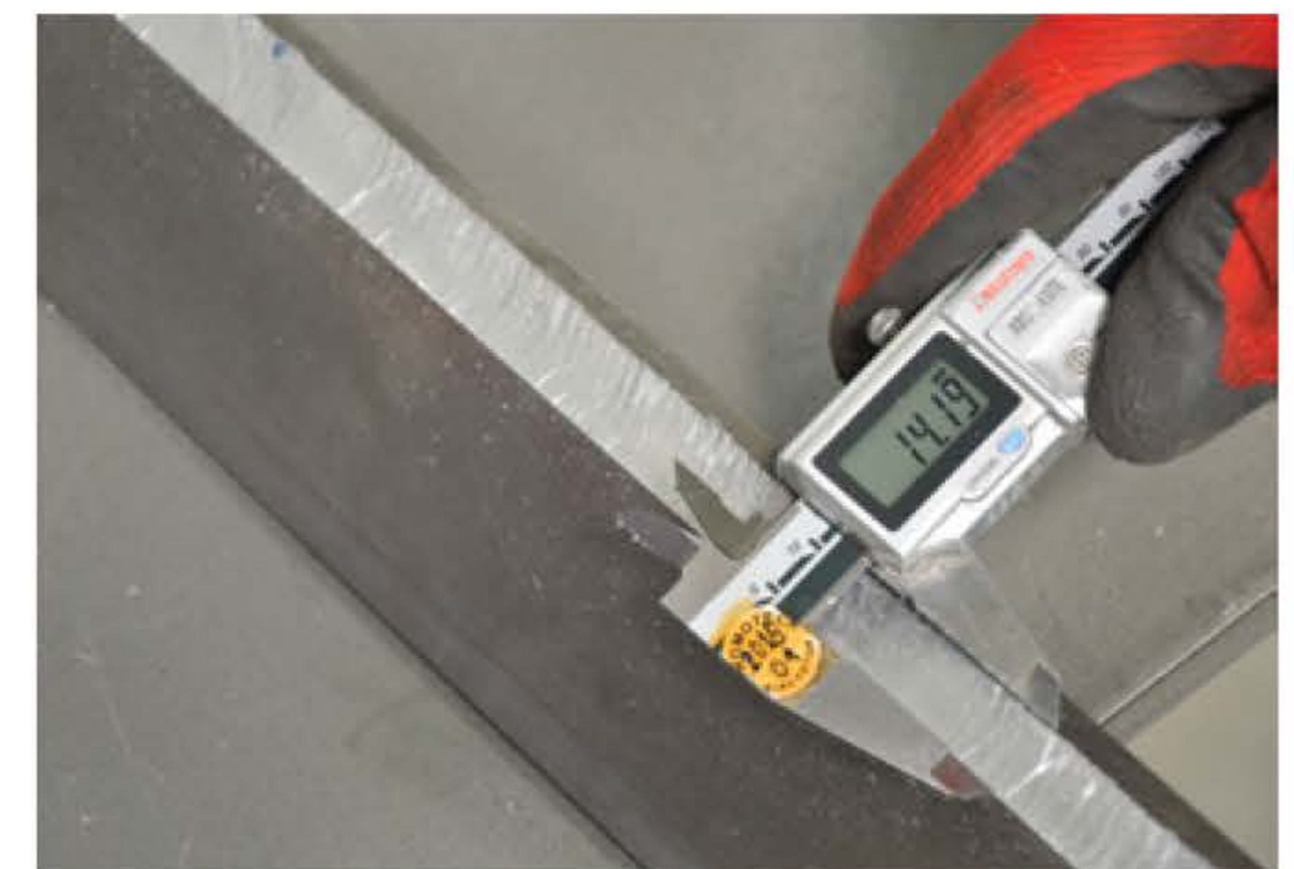
Maximum bevel width up to 14 mm
