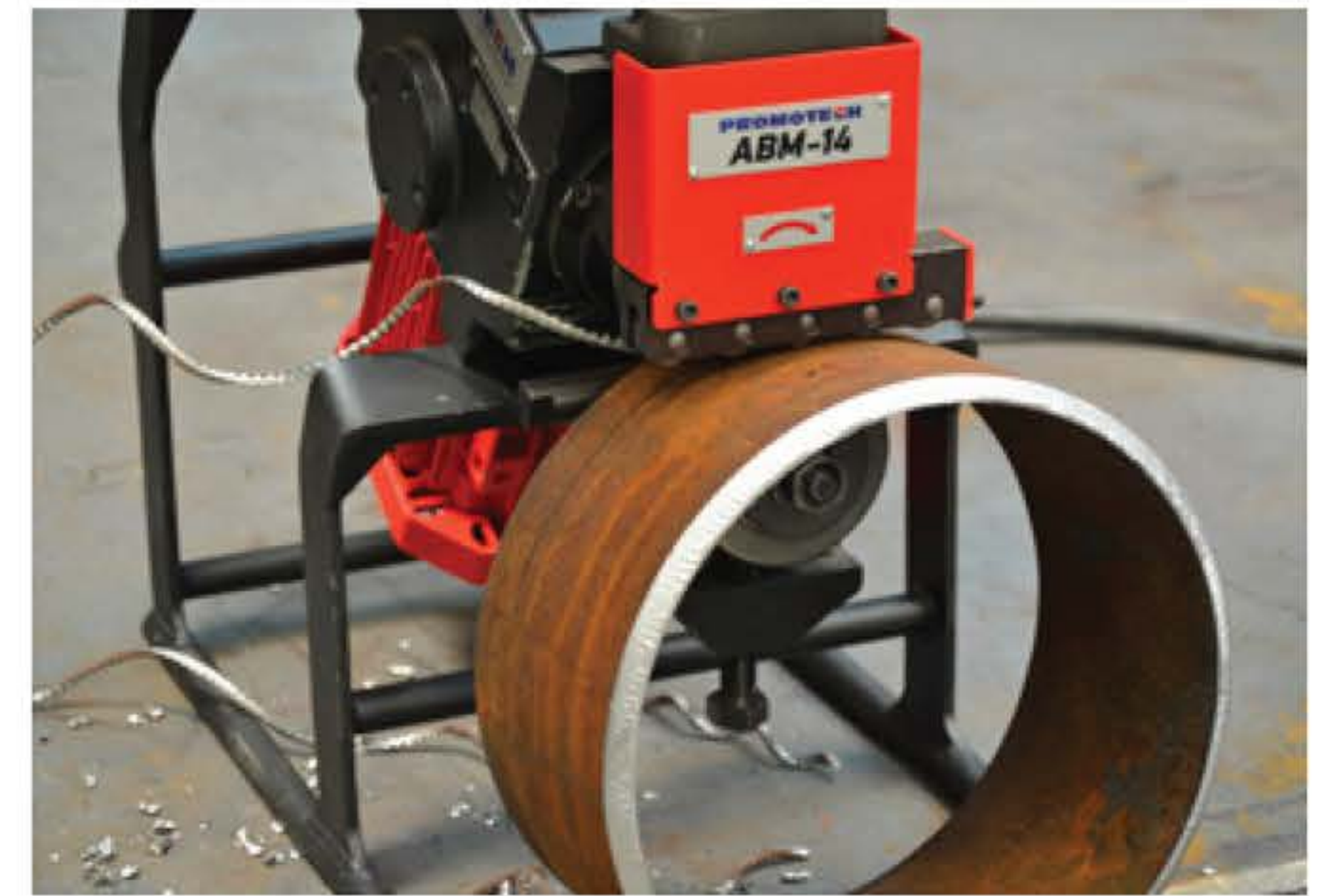
Oval workpiece and pipe beveling
