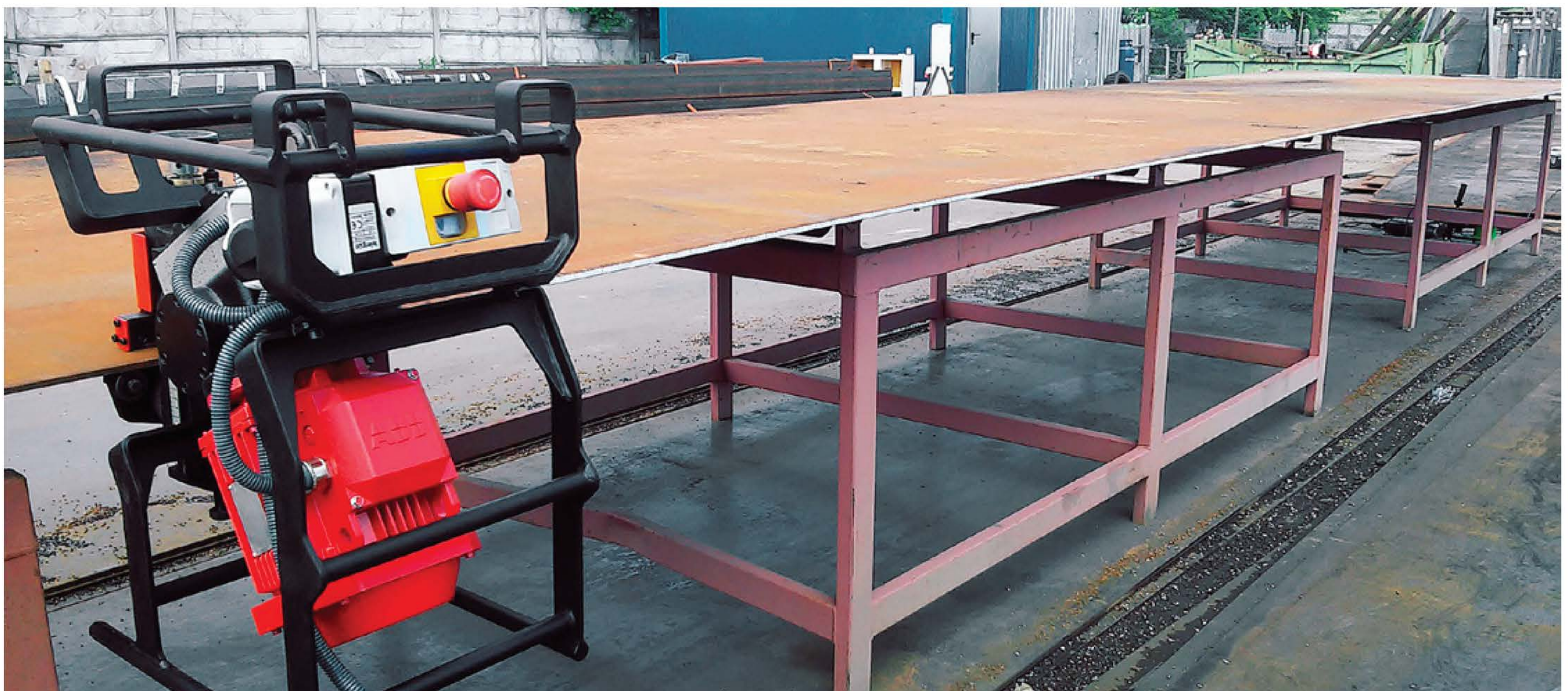
ABM-14 runs along a plate automatically
