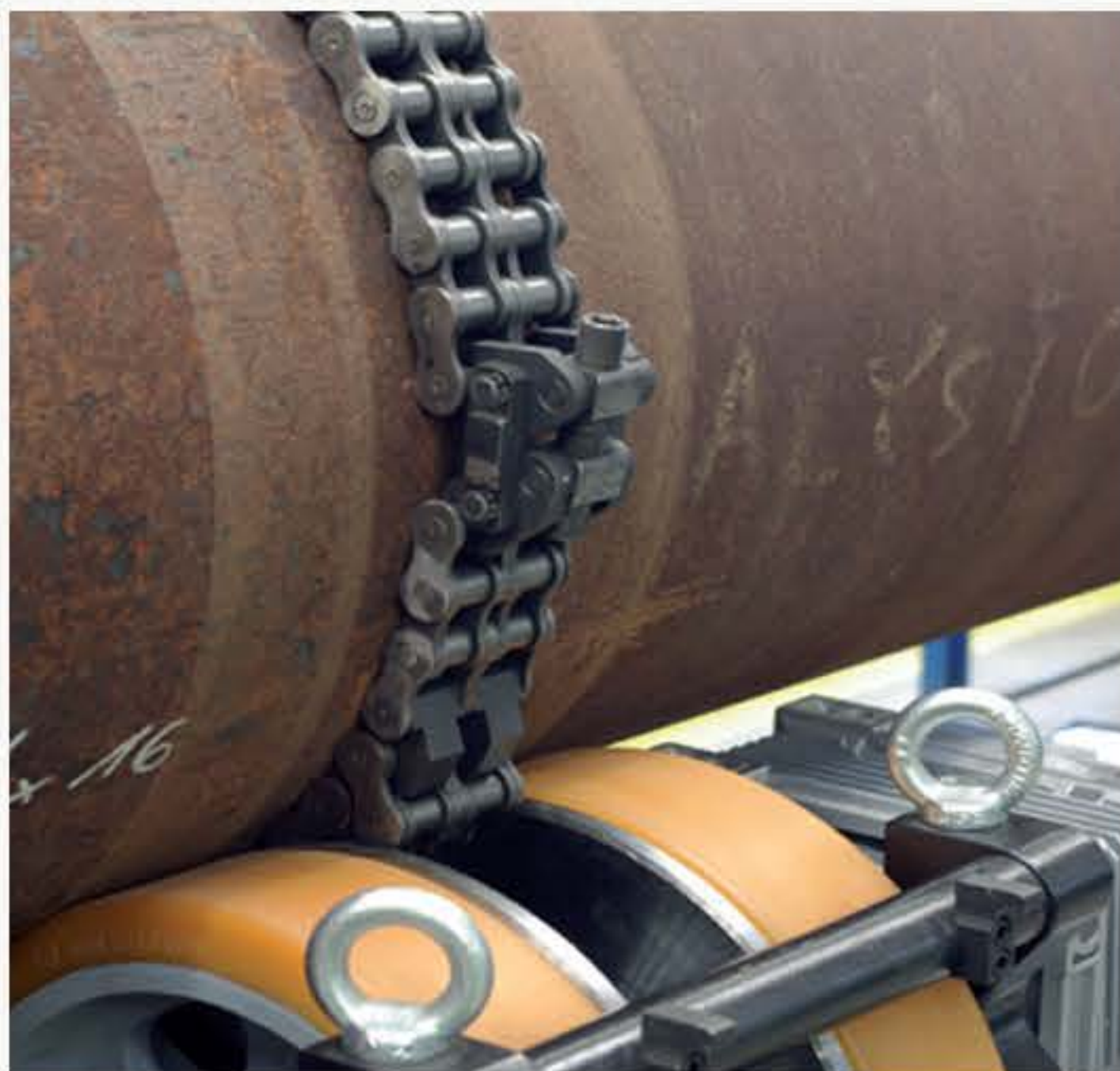
ADJUSTABLE CHAIN (Ø 200-1000 MM) ENSURES POSITIVE AXIAL ROTATION
