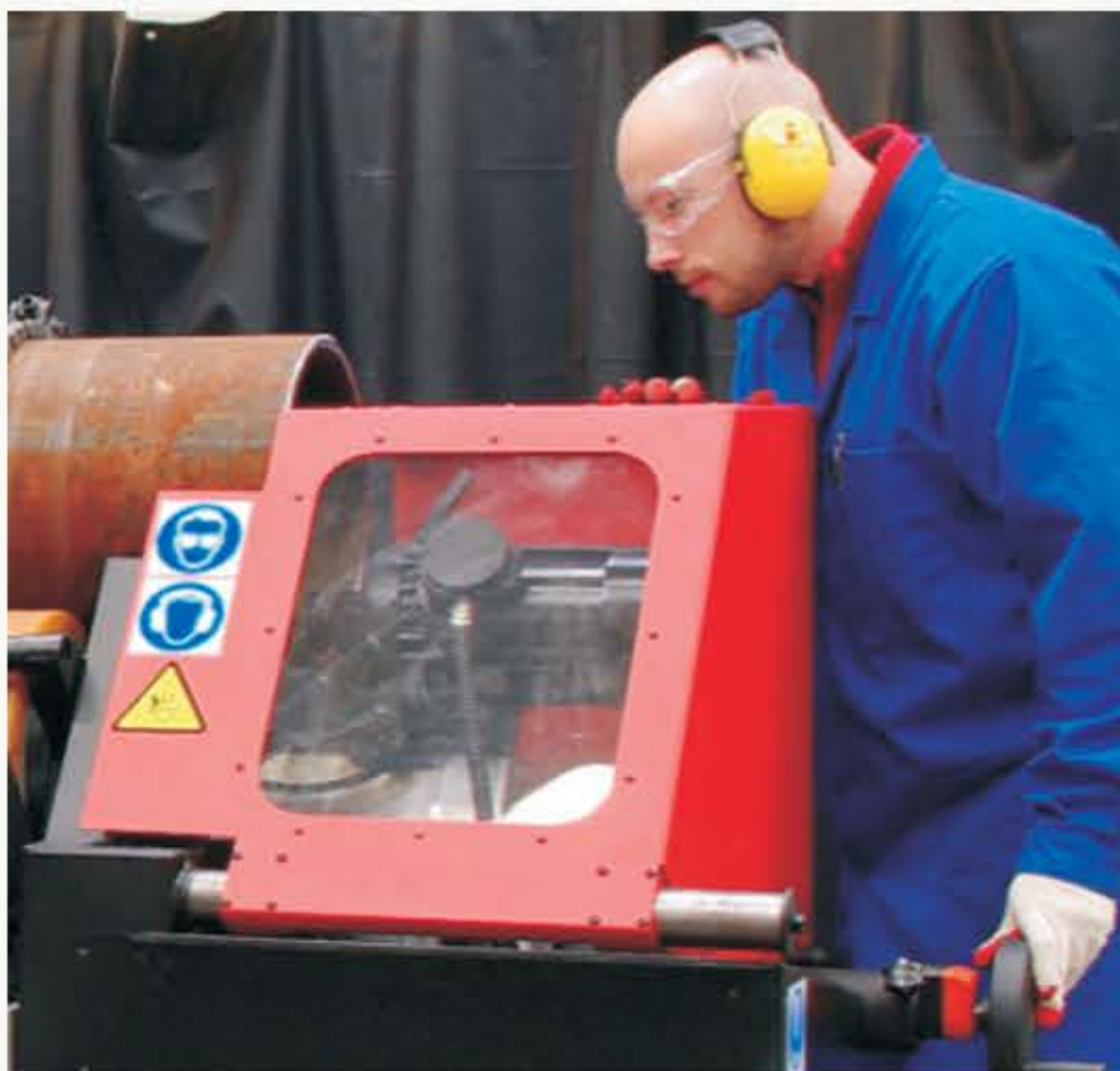
SHIELDS AND INTERNAL LIGHTING INCREASE SAFETY AND COMFORT OF THE OPERATOR
