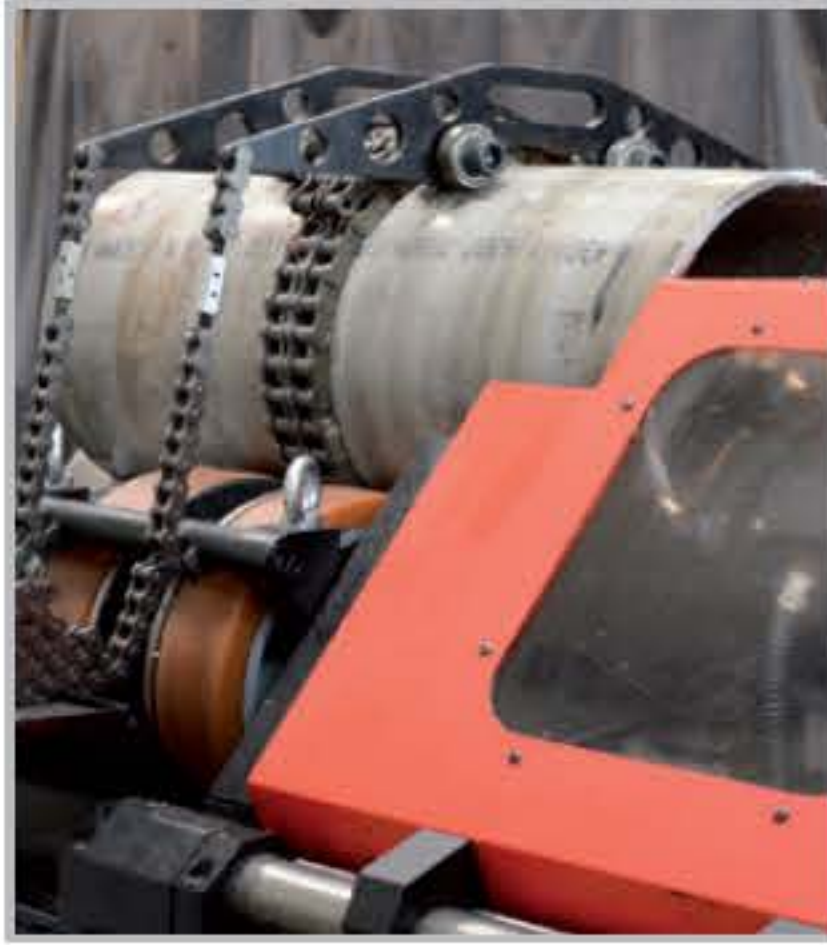
DCS-0436-12-00-00-0 Clamping device for short pipes of 400-830 mm length
