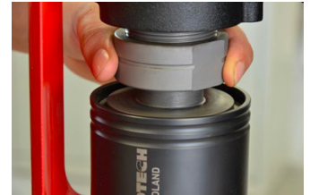
Tapping chuck equipped with securing nut protects tapping tool against pull out
