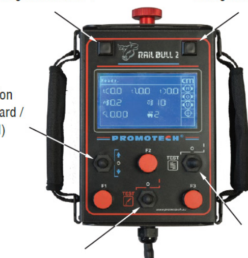
Arc ignition switch (TEST / 0 / I)
