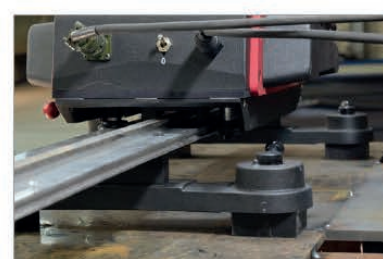
DYS-0482-15-01-01-0 Bracket for Semi Flexible Track
