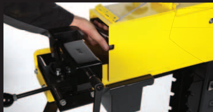
Grinding rollers can be changed without tools.
