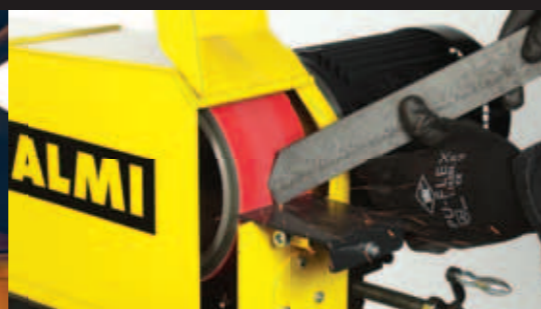
Deburring table on top of the machine Belt grinder on the back
