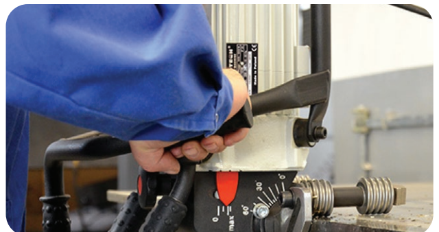
Stainless steel guides for bevelling plate and pipe.
